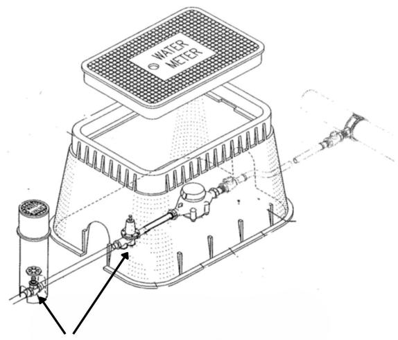
Shut -off valve and pressure regulator installed by Customer
